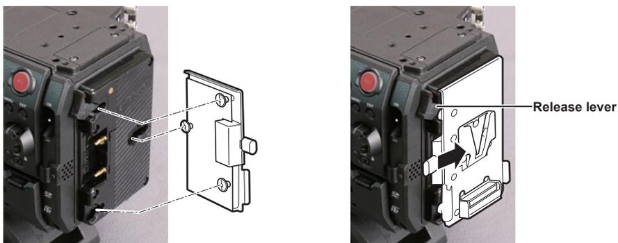
**1** Mount the V-mount type battery plate.
