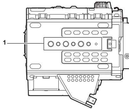
**1 Shoulder mount module/tripod mounting holes**
